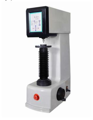
iRock-439T Automatic twin Rockwell hardness tester with a good aesthetic aspect, complete functions, easy operation, intuitive display and good reliability. It is a high-tech product combining the mechanic and electric features, which is suitable to test Rockwell and superficial Rockwell hardness test.
